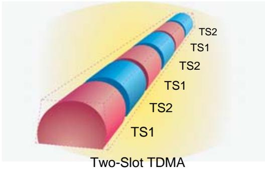
For the amateur, this means one repeater allows two separate channels at the same time. Currently most amateur DMR repeater system implementations utilize both channels for voice and some limited text messaging. Typically one channel (time slot) is used for wide-area and the second is local and regional Talk Groups.
